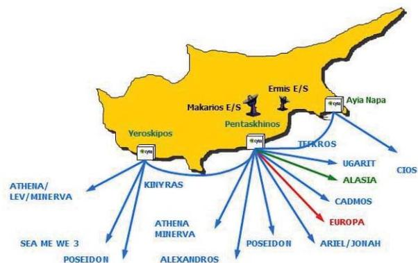
and Egypt and thereafter with the rest of the world. This cable network uses state-of-the-art technology and full restoration and diversity and currently includes the following undersea fibre optic systems that land in Cyprus at three separate cable stations, namely Ayia Napa, Pentaskhinos and Yeroskipos:
