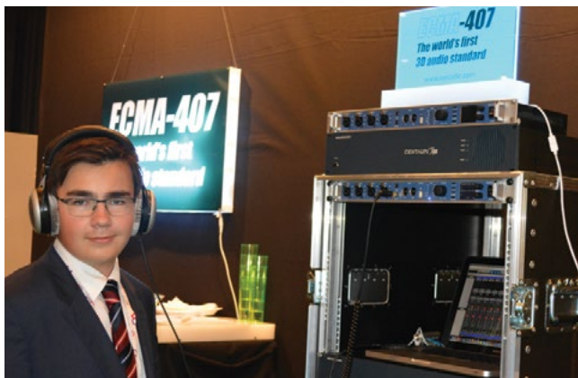
Fig 4: Two ECMA-407 "boxes" in IBC 2014's "Future Zone". Mayah Communication's Centauri-IV 5000 automatically converts HD to UHD audio and encodes and decodes UHD with NHK 22.2 (hidden inside MPEG-4 and Opus as internal multiplex) over an HEVC/MPEG-4 satellite carrier of SES, in real-time . The "Full UHD" program was crafted by France Télévisions.
